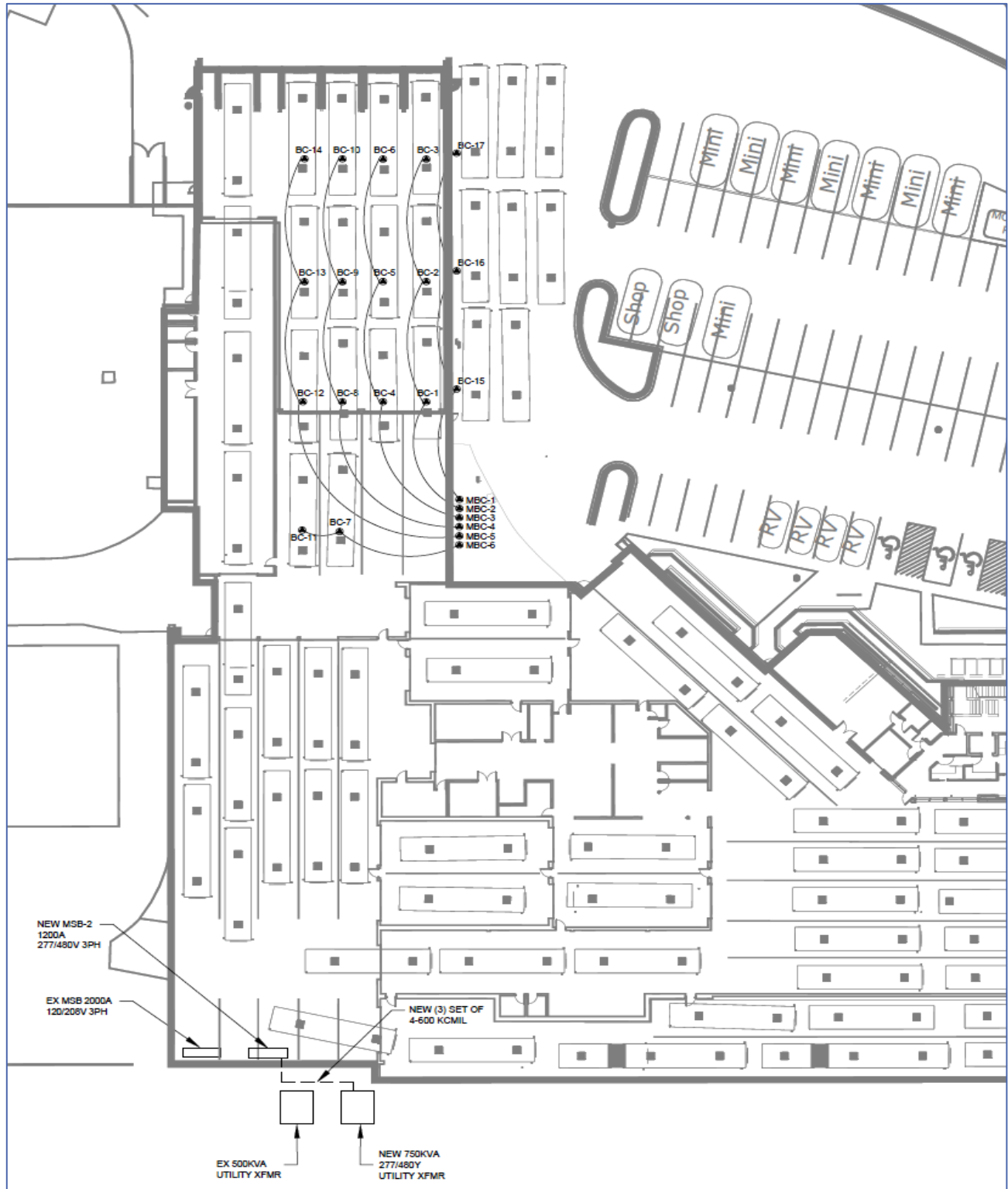
Figure A3-2: Conceptual Charging Design for 17 Buses
